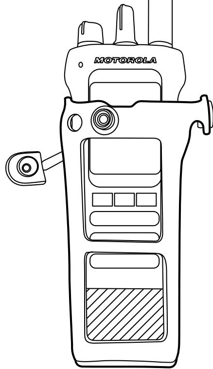
Correct orientation to insert the radio
