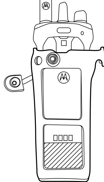
Incorrect orientation to insert the radio
