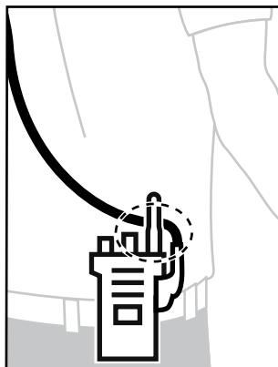
To ensure optimum range and user experience, it is recommended to avoid crossing accessory cable with the radio antenna.
