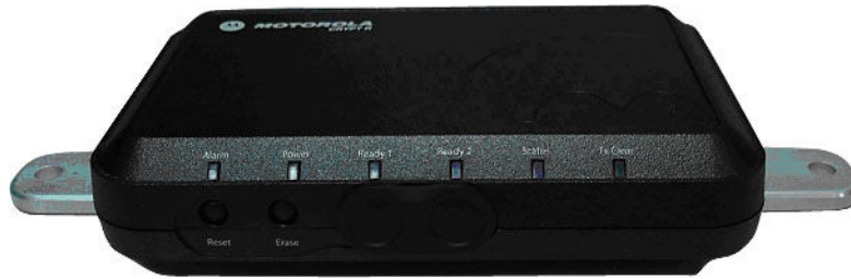
Figure 9: Mounting for Single PDEG Encryption Unit
