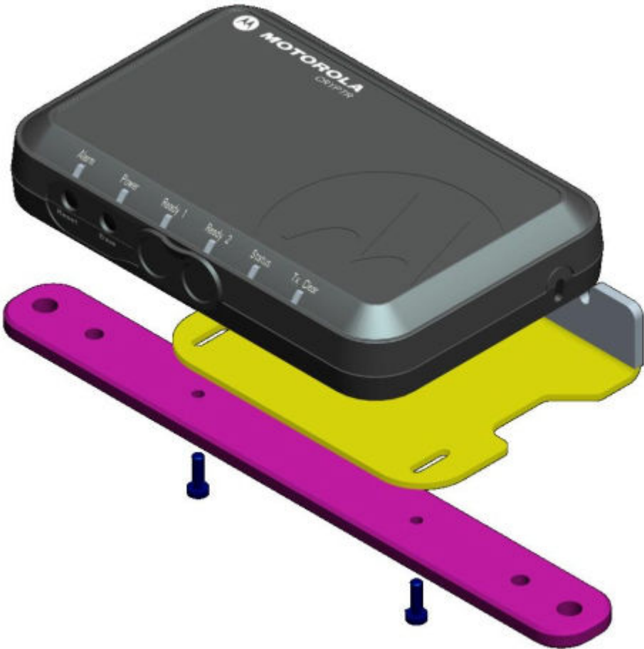
Figure 11: Cable Retention Bracket Mounting
