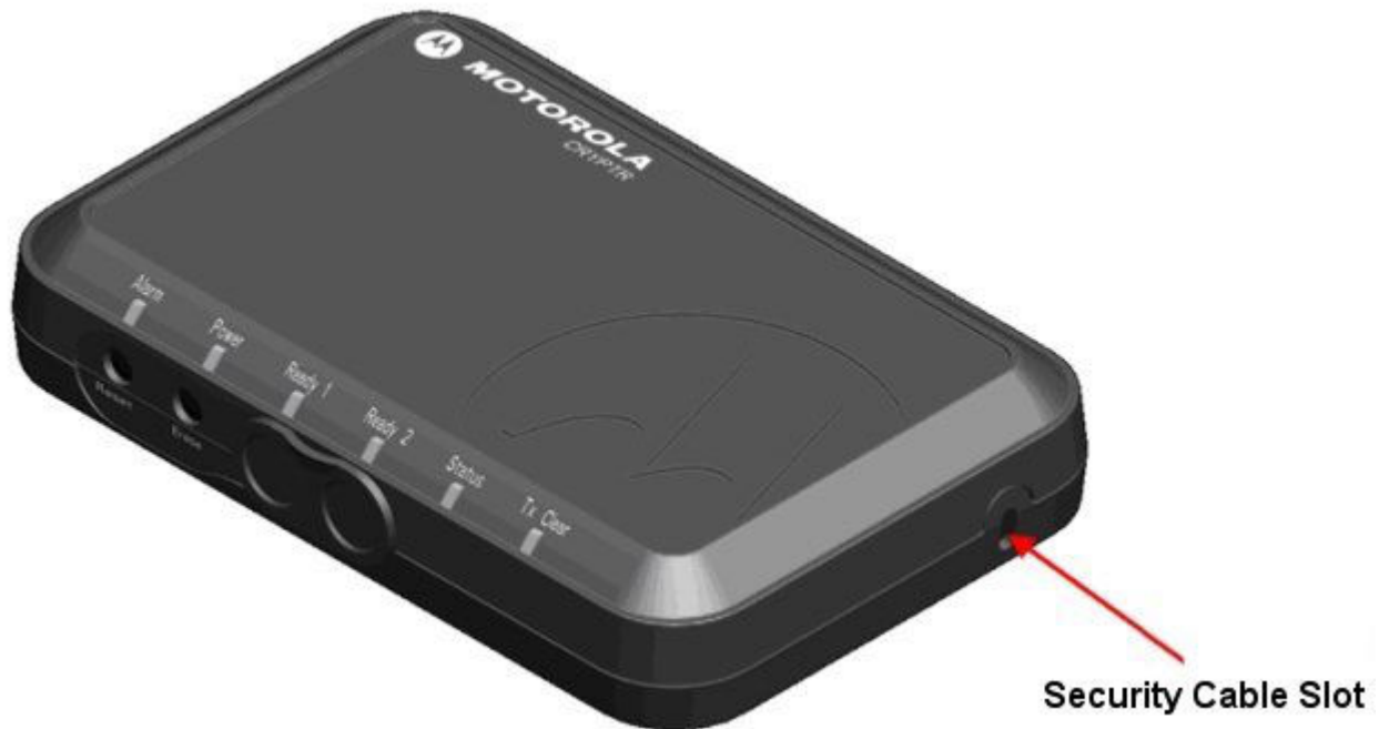
Figure 13: PDEG Encryption Unit Security Cable Slot
