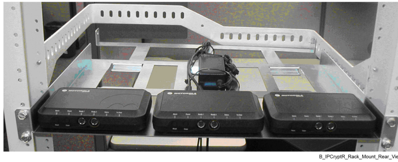
Figure 6: Rear View of PDEG Encryption Unit in Open Rack Mount
