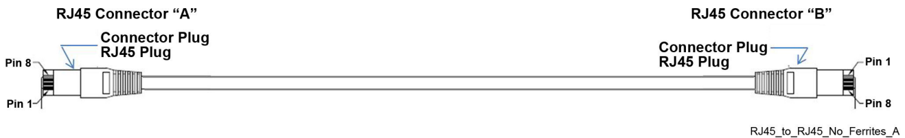
Figure 25: 4W MLC 8000 to GTR 8000 Cable (Non-Simulcast) RJ45-to-RJ45 Cable
