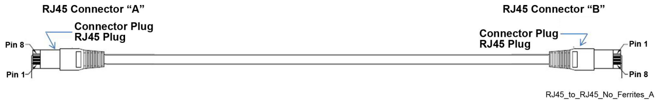
Figure 17: 4W MLC 8000 to QUANTAR Cable (Non-Simulcast) — Option B RJ45-to-RJ45 Cable
