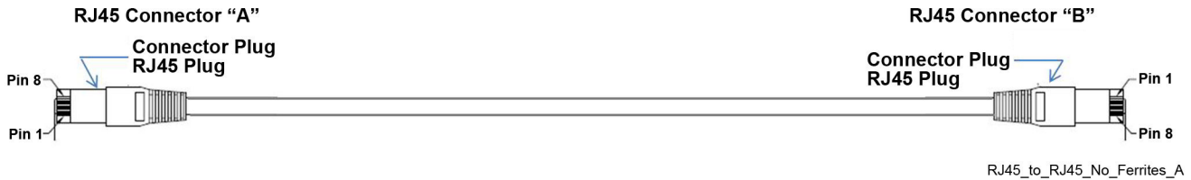
Figure 18: 4W MLC 8000 to QUANTAR Cable (Non-Simulcast) — Option C (RJ45-to-RJ45 Cable)
