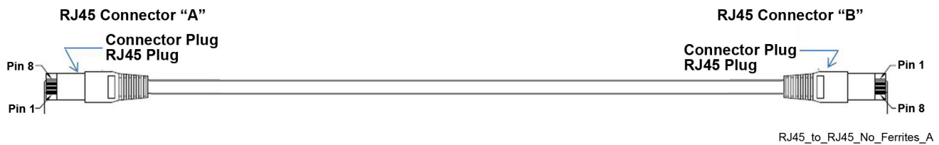
Figure 34: 4W MLC 8000 to Channel Bank Cable (Circuit-Based Non-Simulcast Voting) RJ45-to-RJ45 Cable
