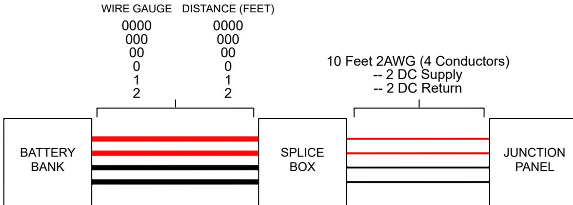
In some installations, local codes may require the installation of wire heavier than 2 AWG. In these situations, a local splice box can be used to reduce the incoming wire to the 2 AWG needed for connection to the input terminal box. The splice box should be as close as possible to the junction panel.
