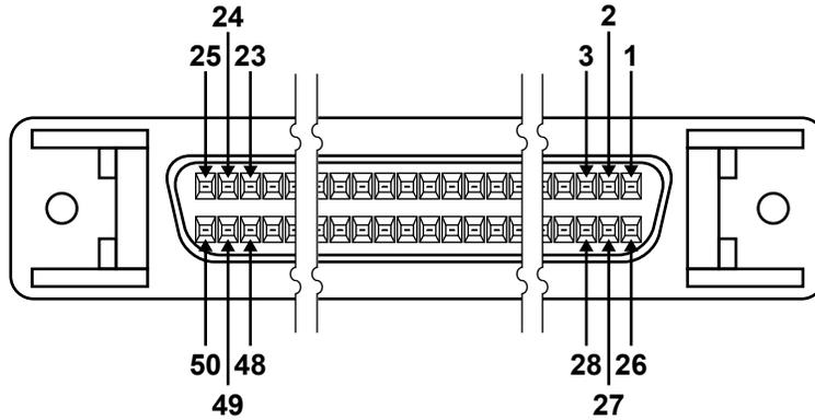
Table 39: 50-Pin System Connector Pin-Outs (Conventional)
