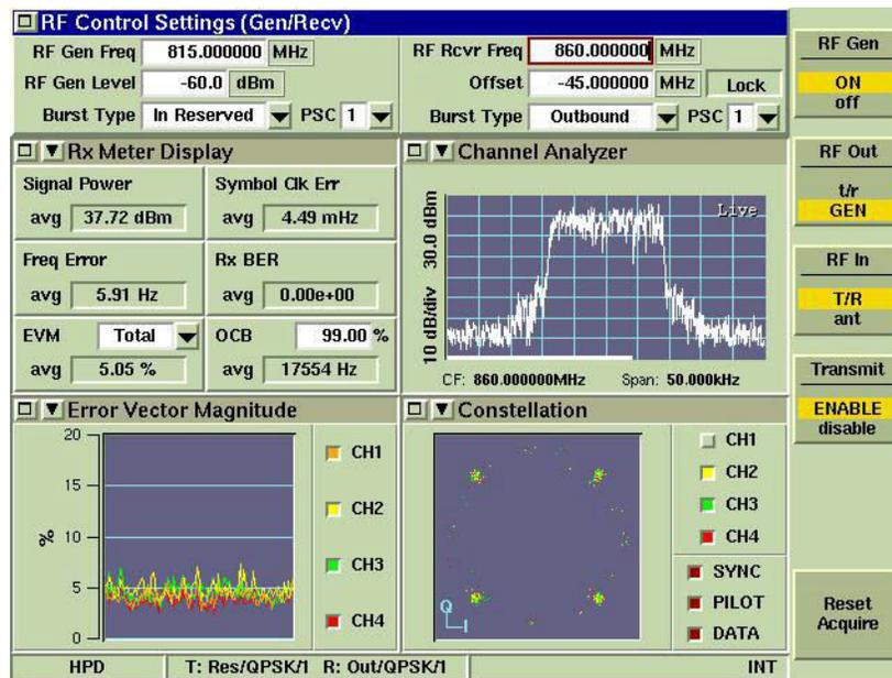
The HPD Service Monitor is connected with an HPD base radio to perform the following diagnostic tests (for additional tests, see the HPD service monitor manual). These tests determine whether the equipment is operating within specification. If the HPD base radio fails to meet specification, service may be required.
