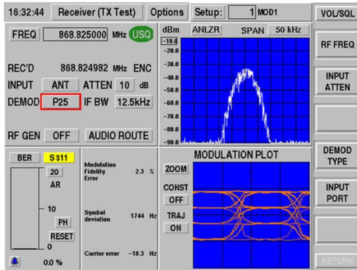
7. Record the Bit Error Rate (BER), Modulation Fidelity Error, Symbol Deviation, and Carrier Error and FREQ readings from the P25 Uplink Data (in the Options menu) for use in digital Receiver Testing.
