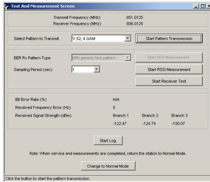
9. Set up the **Test And Measurement Screen** to display received Bit Error Rate (BER):
