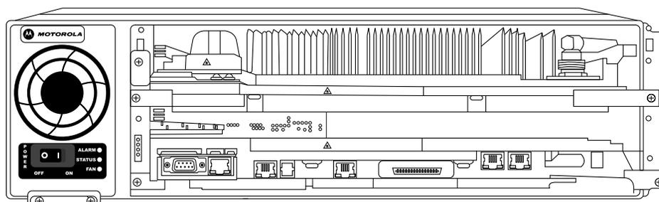
**NOTE:** The IP address for the device is available through a serial port connection in Configuration/Service Software (CSS) in the **Tools** menu.
