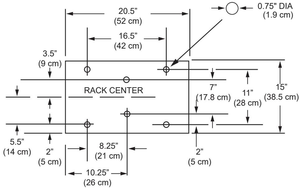
Figure 38: Open Rack – Side View
