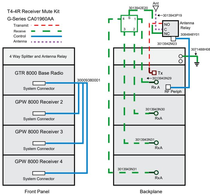
Tn-nR Receiver Mute configuration option kit is used with a standalone GTR 8000 Base Radio and up to three GPW 8000 Receivers.
