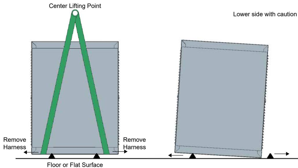
2. Using the harness, lift the cabinet onto the two supports.
