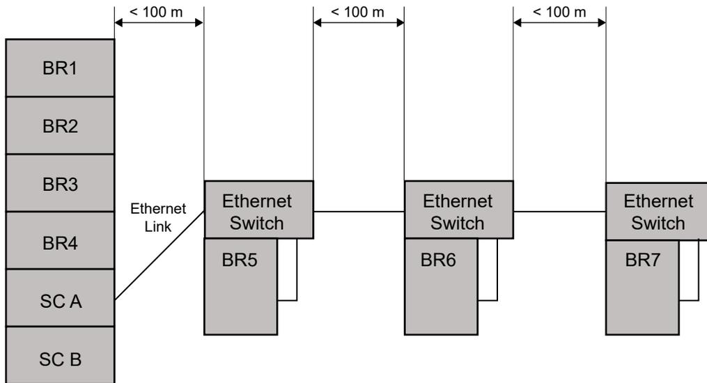
If the distance between the first non-colocated base radio and subsequent non-colocated base radios is less than 328 ft (100 m), a single Ethernet LAN switch can be used to distribute the site controllers call control signaling to those non-colocated base radios. The stated distance limit for a shielded twisted pair Ethernet cable (CAT5) is 328 ft (100 m) before the signal degrades too much to be used.
