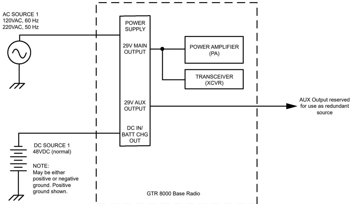
If present, the base radio operates from AC power as the preferred power source. When AC power is not available, the base radio switches to operate from the DC source. Operation returns to the AC source when the AC source is restored. Switchover from AC to DC and back again is fully automatic.
