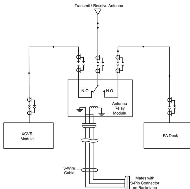
Figure 30: Functional Block and Interconnect Diagram for Antenna Relay Module (Peripheral Tray Mounting)
