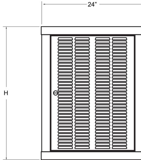
Figure 36: Cabinet Dimensions – Side View
