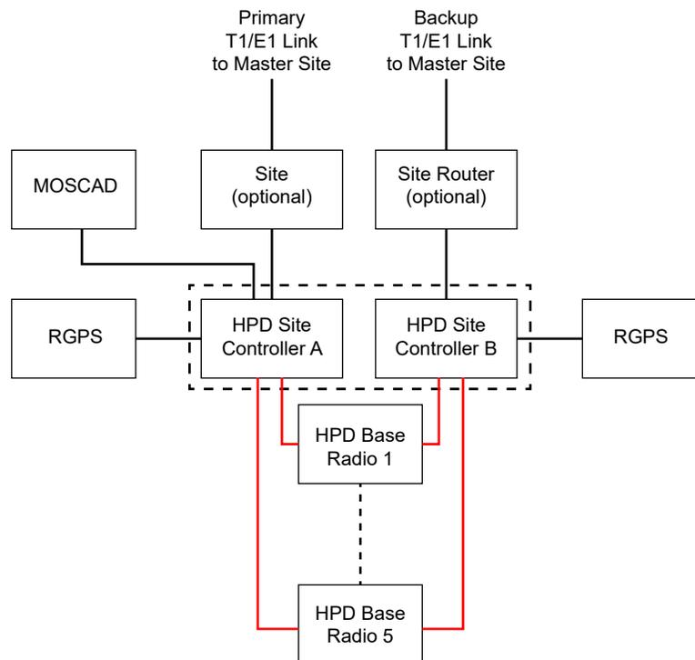
The HPD base radio uses Time Division Multiplex (TDM) frames for random access channels, reserved access channels, and broadcast messages. All carriers in the system are synchronized by a Global Positioning System (GPS) so that transmission slots are synchronized across sites. The base radio is able to schedule inbound/outbound traffic for half-duplex MSUs so that outbound traffic intended for the MSU does not conflict with inbound random or reserved access traffic from the MSU.
