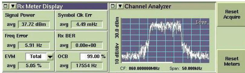
9. Compare the value displayed in the **Signal Power** field to the base radio Tx Power Out specification that matches your base radio configuration.
