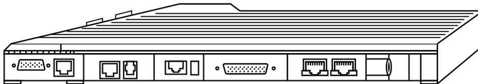
The transceiver generates the station reference, which typically must be locked on to one of many possible external sources. The external source can be either the site controller TDM clocks or the external reference operating at 5 MHz or 10 MHz.
