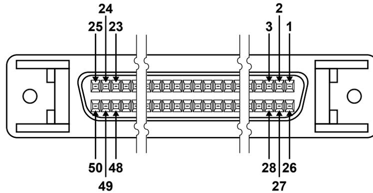
Table 40: 50-Pin System Connector Pin-Outs (Trunked 3600)
