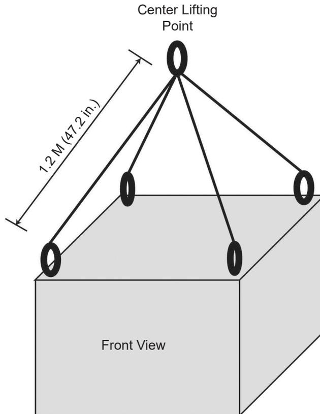
If eyenuts are removed or become loose, install them properly before lifting the equipment rack. Tighten the eyenuts and bolt assembly by hand. Correct eyenut tightness and alignment are crucial to ensure that the
