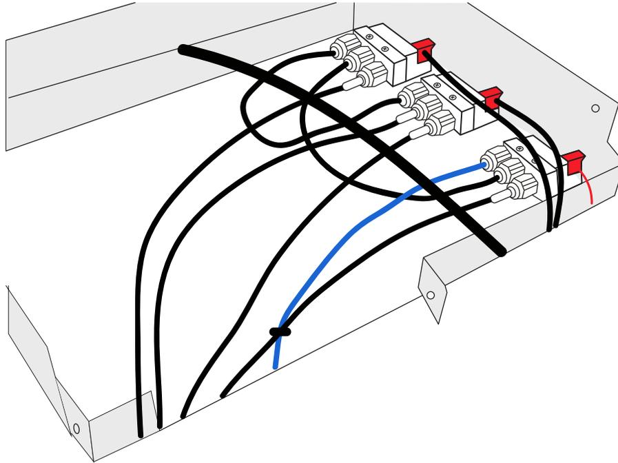
**Figure 131: T2-2R with Duplexer and Triple Relay Option Kit Wiring**
