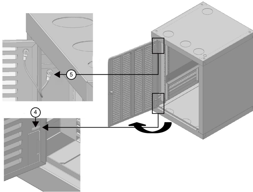
4. Flip the door 180° and reattach it to the cabinet with the pin hinge.
