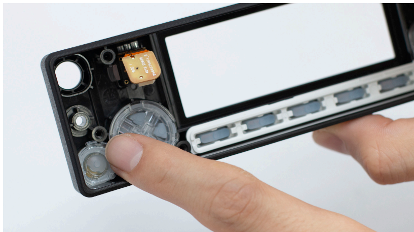
Figure 66: Home Button [14] and Home Button Retainer [15]
