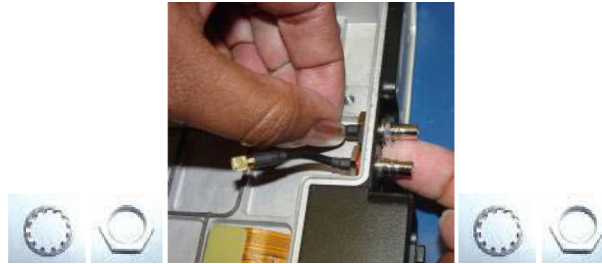
Figure 82: Installing QMA Lock Washer and QMA Nut for each cable connector
