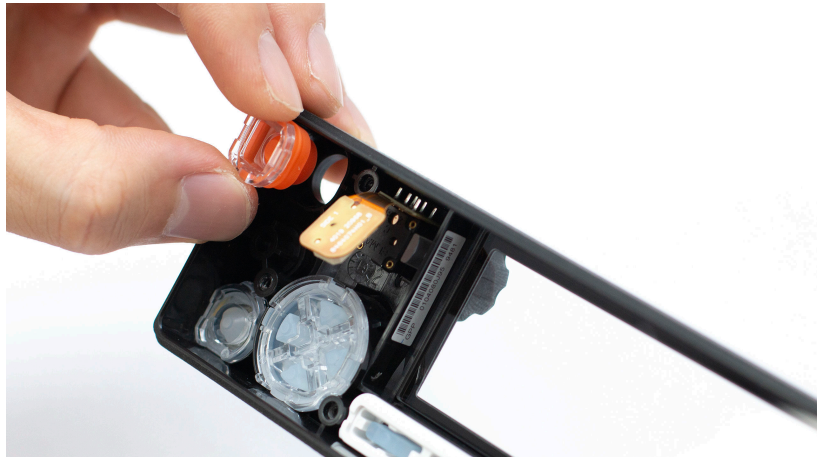
Figure 66: Home Button [14] and Home Button Retainer [15]
