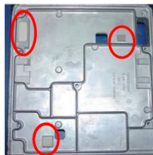
Figure 77: Location of the Thermal Pads on the Transmitter (TX) Side of the Main Chassis
