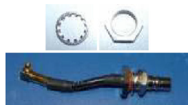
Figure 80: Removing the QMA Lock Washer and QMA Nut
