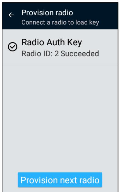
Next radio may be connected to the KVL and after pressing 'Provision next radio' button KVL application goes to the next screen where a user can enter a key value again.
