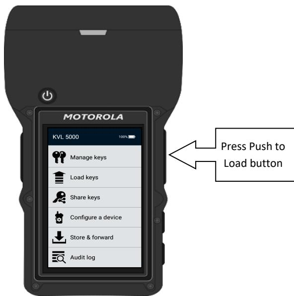
If this is the first time you are loading keys (or previously loaded keys were removed from KVL), push the PTL button and you will be moved to Select keys menu. You can go back to your previous screen by pressing back button.
