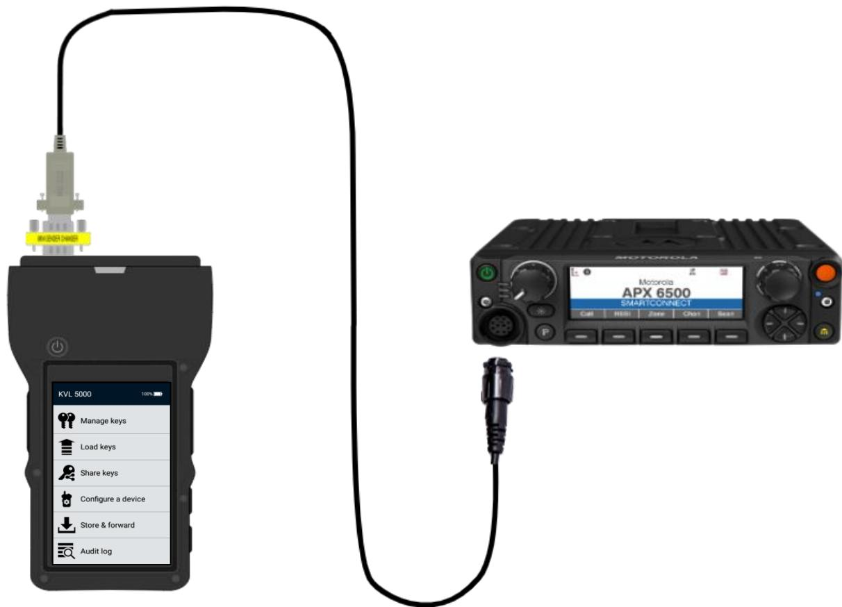
You can also load authentication keys to mobile radios over control head using serial cable.
