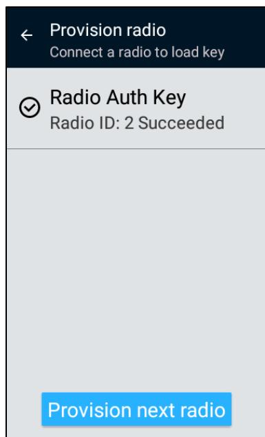
Next radio may be connected to the KVL and after pressing 'Provision next radio' button a new radio authentication key will be generated and loaded to the radio.
