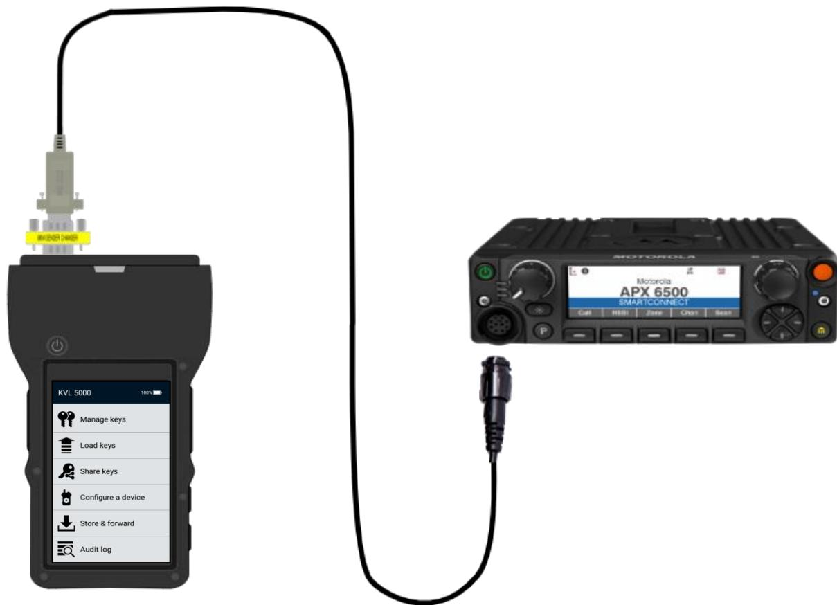
You can also load keys to mobile radios over control head using serial cable. To do that you must first [Provision mobile radio with control head keys](#)
