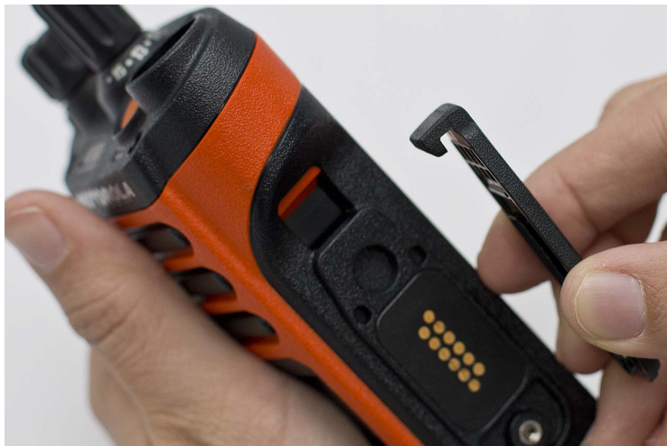
Figure 7-8. Pull the Accessory-Connector Cover away
