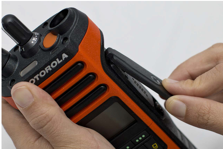
Figure 7-7. Lift the Accessory-Connector Cover
