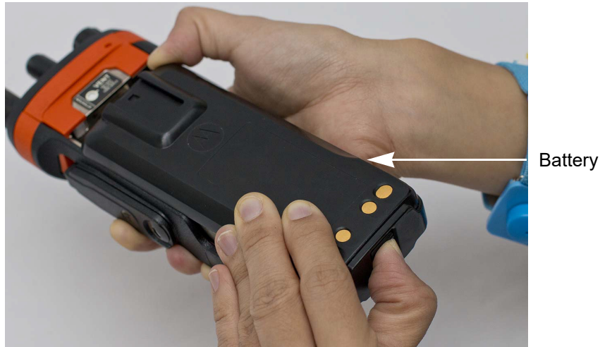
Figure 7-13. Reattach the Battery – Slide into Position
