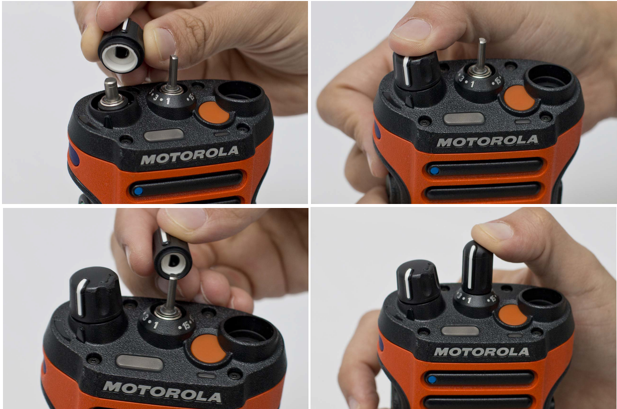
Figure 7-11. Reassemble the Volume/Channel Knob
