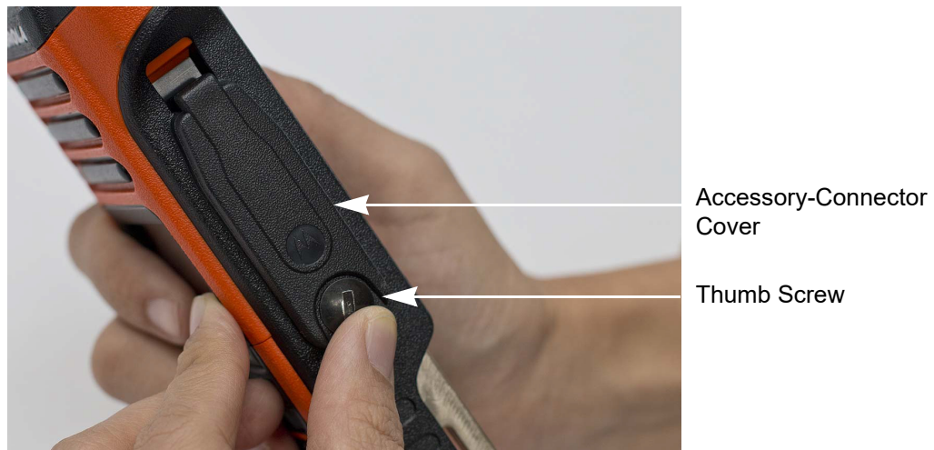
Figure 7-6. Removing the Thumb Screw
