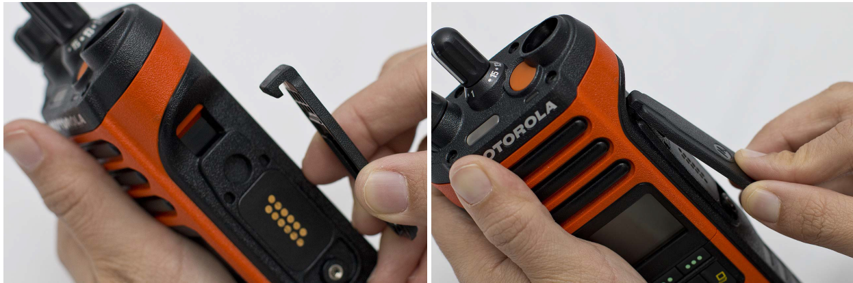
Figure 7-9. Reassemble the Accessory-Connector Cover
