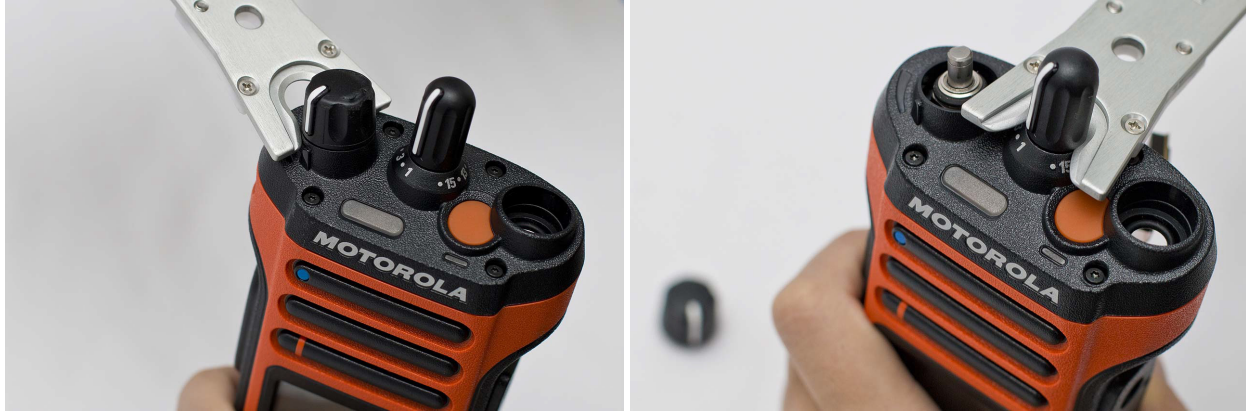
Figure 7-5. Removing the Volume/Channel Knob
