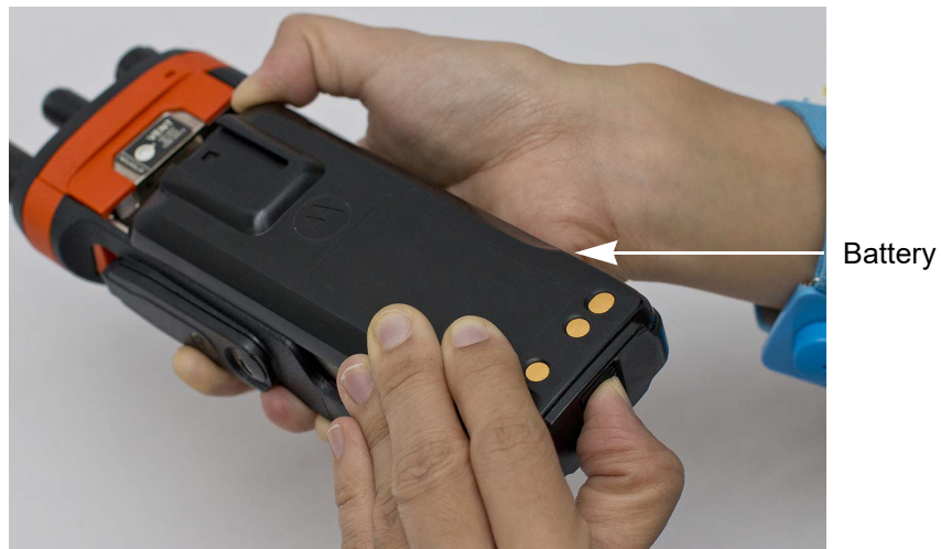
Figure 7-3. Removing the Battery
