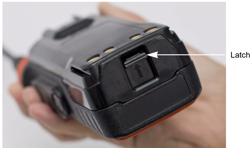
Figure 7-2. Lifting up the latch
