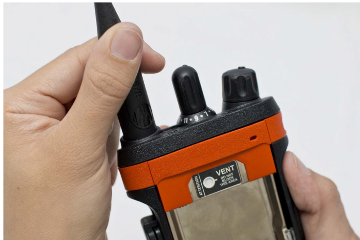
Figure 7-12. Reassemble the Antenna
