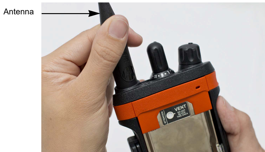
Figure 7-4. Removing the Antenna
